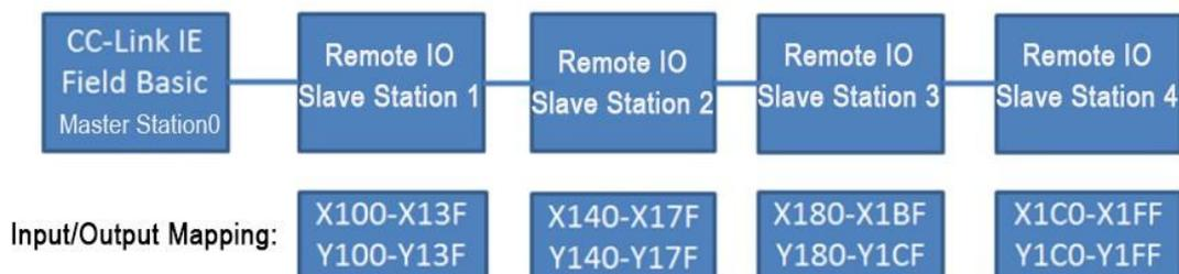
Fig. 5-3-10 Slave Station IO Point Mapping
