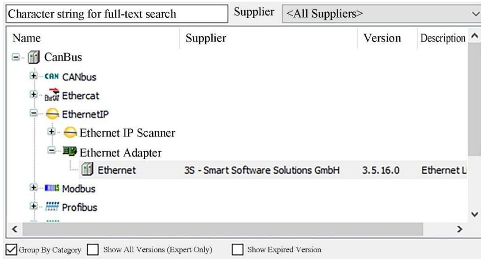
Fig.5-7-21 Add Ethernet Adapter
